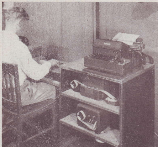
PAPER TAPE is punched on standard equipment used in teletypewriters. Operator follows code directions, in which blueprint lines have been changed to column of figures.
